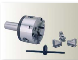
B90-AF01B (to be used with B90-C2SH ) 4" Adjustable 3-jaw Chuck mounted on B&S NO.11 taper arbor which will fit all fixtures with B&S NO.11 spindle.
